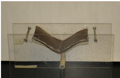
Figure 10. Experimental apparatus to study oropharyngeal fluid mechanics.
