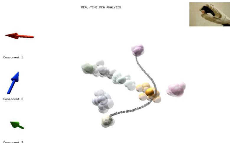
Fig. 3.8: Observation of the targets and their data cloud in the projected space. Top right picture shows the hand pose represented by the highlighted cloud (in orange). Transparent spheres are the recorded positions; solid ones correspond to clouds' means.
